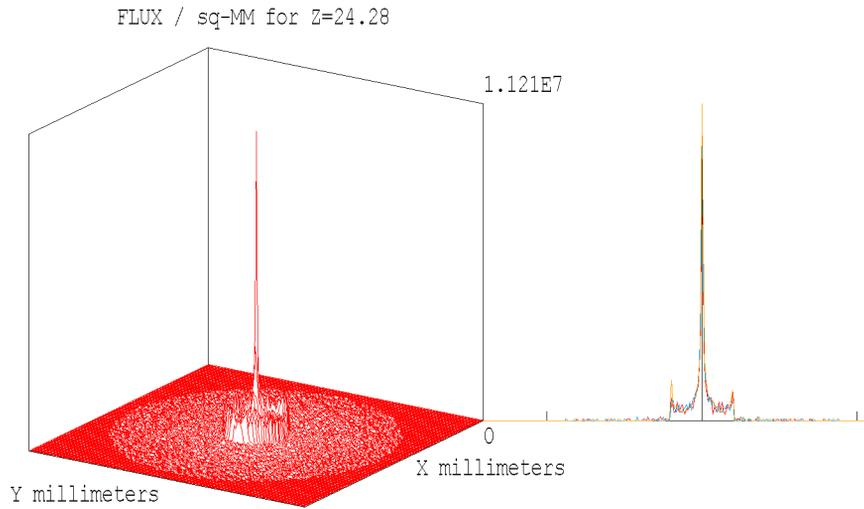
Figure 8 Isometric view of the retinal image PSF constrained by retinal window dimensions (left), and overlaid retinal image PSF X and Y cross-sections (right)
