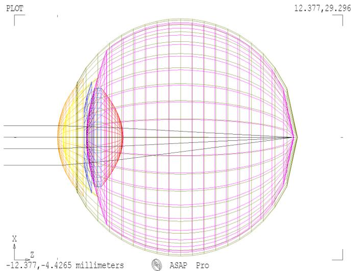
Figure 6 Cross-section of advanced human eye model. Default faceting level set low at 5 for high-speed rendering.
