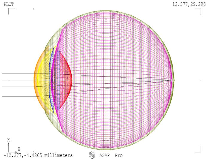
Figure 7 Same system as in Figure 6 but with level 15 faceting. Higher faceting, which takes slightly longer to render, produces a smoother and rounder graphic.
